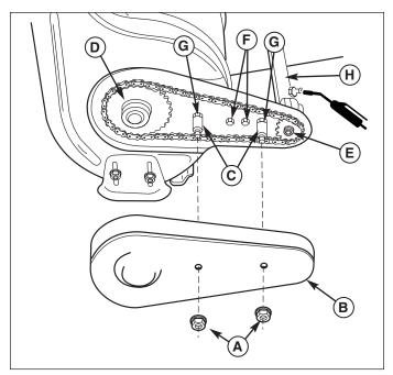
Figure 3. Drive Chain Lubrication & Adjustment
